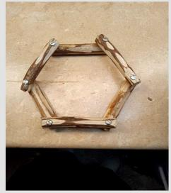
Step 3: Screw smaller extension cuts to the ends of each bottom piece facing outward.
